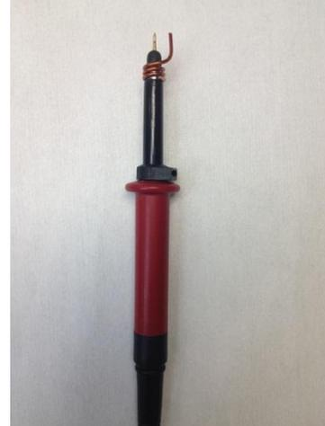
Fig.6. Typical probe with 3-inch ground lead – should not be used      Fig.7 Probe with short ground lead – should be used
