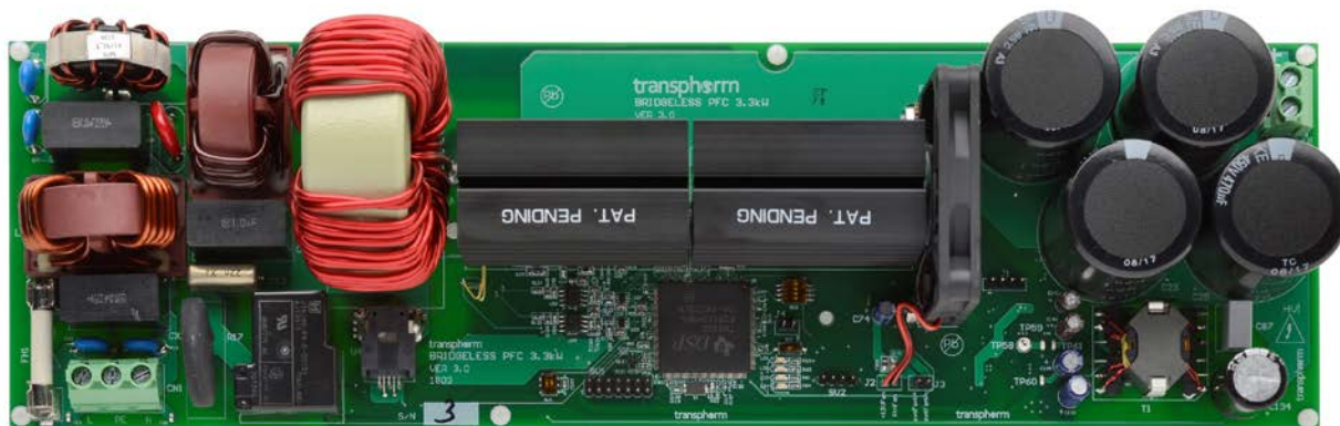
Firmware-based 3.3kW bridgeless totem-pole PFC reference design demo board
